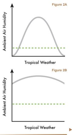
Desiccant dehumidification can bring air humidity down with at least 12g/kg, for example from 14 to 2g/kg or from 22 to 10g/kg in one step without any use of chilled water. Figures 2A and B show how the ambient air humidity is controlled at constant levels in both temperate and tropical climates.
